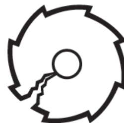
Inspect jammed blade for damage
