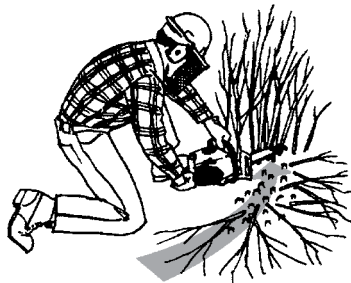
KICK GUARD® ALLOWS SCYTHING ACTION TO REMOVE BRUSH
