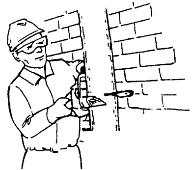
KICK GUARD® ALLOWS KICK-BACK FREE CUTTING NEAR MASONRY, FENCES, ETC.
